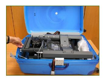
The 10 Kg. **Traveller**, including the lighting system, collapses and fits into the case provided measuring approximately 82 x 57 x 33 cm.
